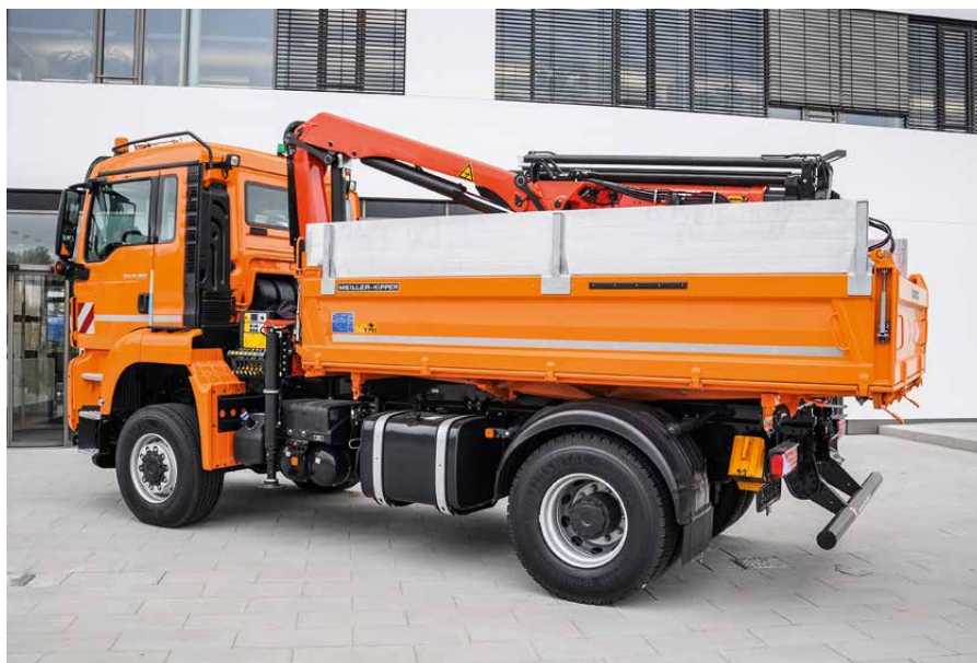
MEILLER three-way tipper type 9 prepared for loading crane and aluminium extension walls
