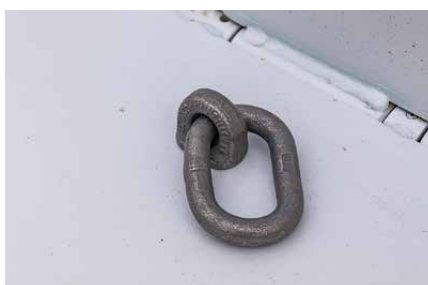
The lashing lugs in the corners of the floor (with 8 t lashing capacity) allow for variable securing possibilities.
