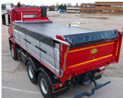
MEILLER side roller tarpaulin must be operated from below with a crank.
