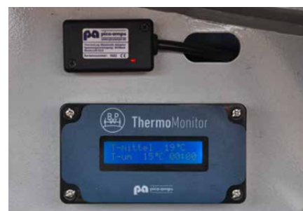
Measurements are made every minute: a transport log monitors the quality of every load.
