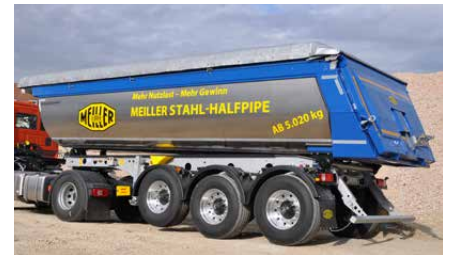
Insulated tipping semi-trailer with MHPS half-pipe steel tipping body
