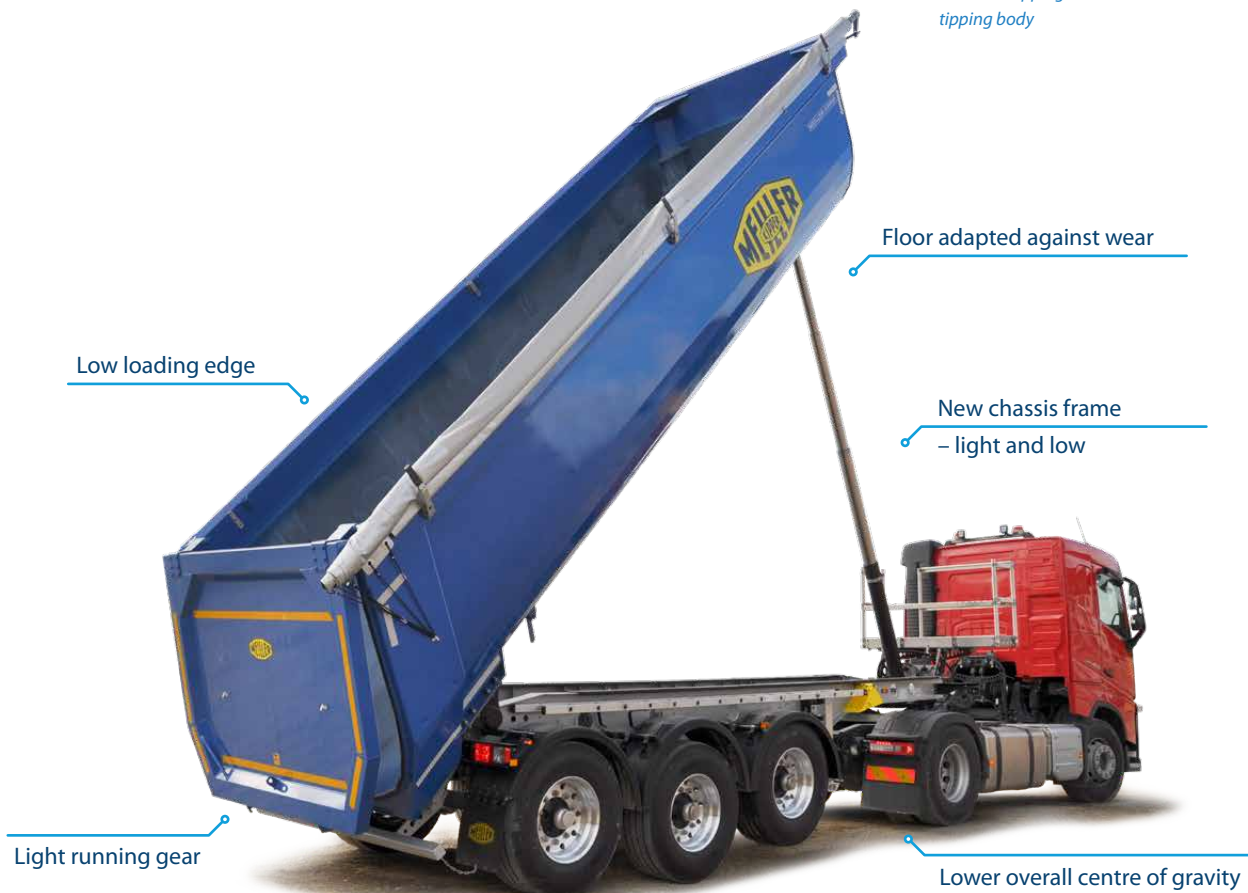
Insulated tipping semi-trailer with MHPS half-pipe steel tipping body
