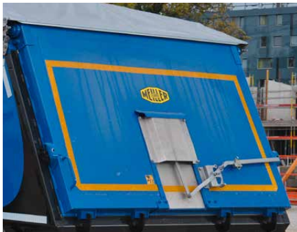
Secure locking and perfect dosing with the grain slider.
