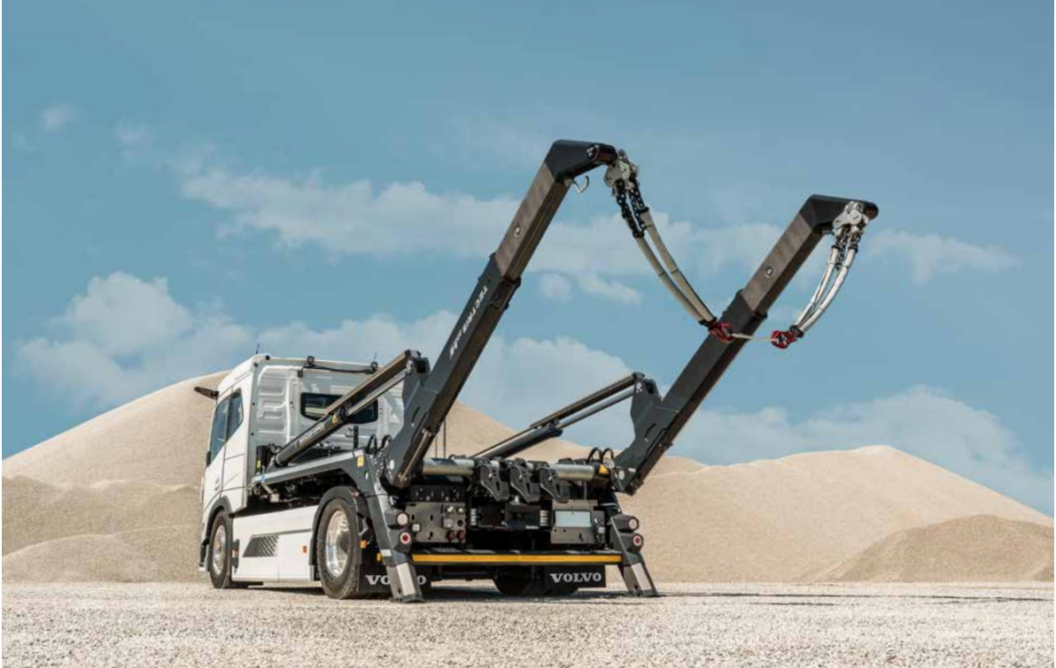
The telescopic equipment achieves long reaches of almost 4.5 metres, e.g. for easy transfer of the skip in trailer operation.
