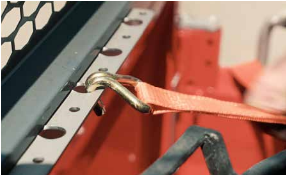
Side and front wall lashing eyes also for transporters and light 2-axle vehicles
