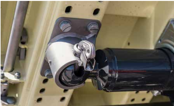
Ball-type tipping parts for one-hand operation
