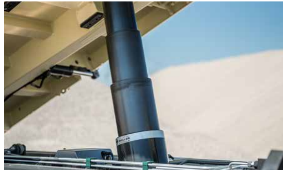
Only one hydraulic telescopic cylinder on the 4-axle vehicle
