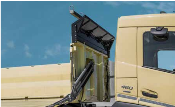
Folding with spring load relief system
