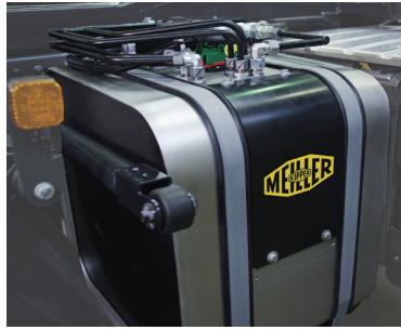
Everything from a single tank: Several consumers (tipper, crane & hydraulic system for municipal services) can be supplied from one compact MEILLER tank.
