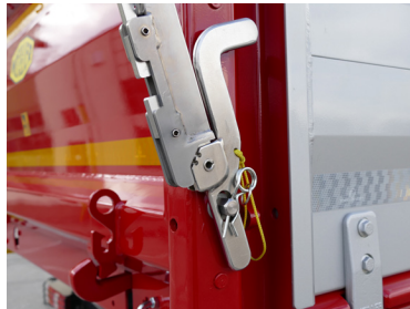
Legally compliant operation: The maximum outer width is adhered to with the flat crank.
