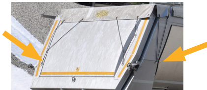
Tensioning without operating hooks due to low-lying hooks. The side flap ensures elasticity when tilting into a road finisher.
