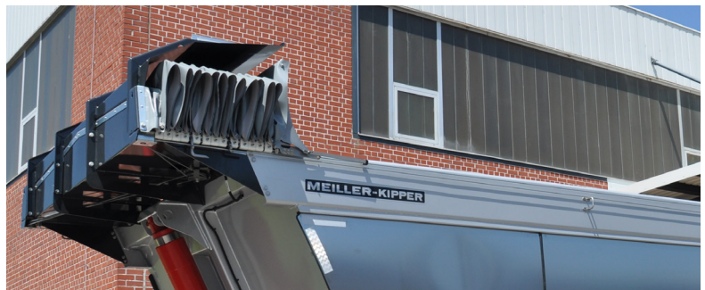
Tarpaulin protection roof protects during loading.
