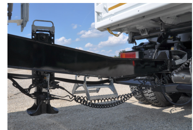
The climb-over on the tow bar with handle on the stabilising leg facilitates the opening and closing of the side roller tarpaulin on the centre-axle trailer.
