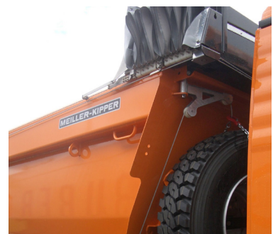
MAXTREME: spare wheel on the front wall.
