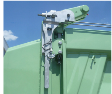
Three-way tipper: Detachable cables due to quick-release fastener.
