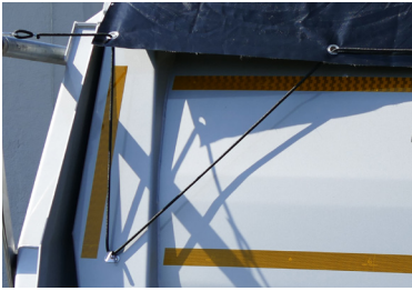
MAXTREME: Tensioning is easy to handle due to low-lying hooks.
