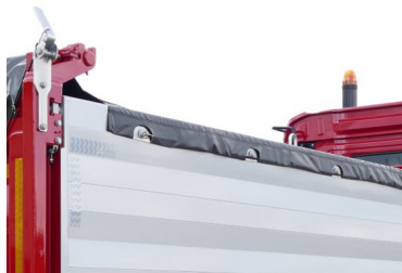
An eccentric bearing on the top belt of the tipper body allows the retensioning of the side roller tarpaulin.
