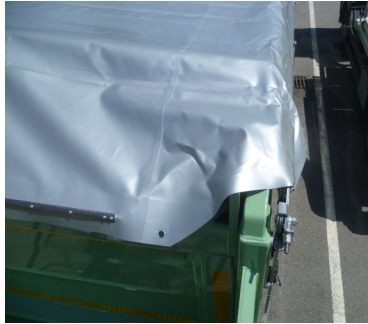
Three-way tipper: Tarpaulin fully covers the tailgate bearing.
